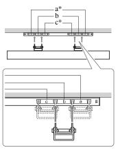
Hook location "a" and "c" cannot be used for the models.
